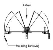
□ VCR8 - Steel full flow damper, duct mounted (sizes 6" to 14")
