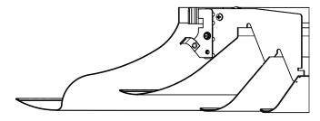
□ RCD - adjust by repositioning cone mounting brackets
